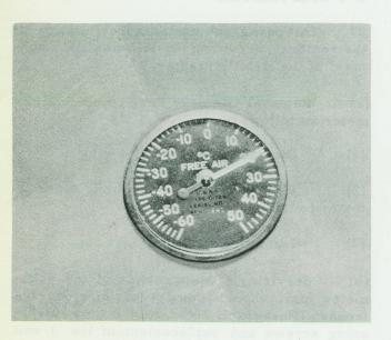
Figure 6-5 Outside Air Temperature Indicator
