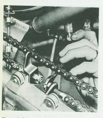
Figure 2-73 Landing Gear Chain Adjustment
