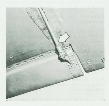
Figure 2-41 Elevator Tab Travel Adjustment
