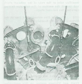
Figure 5-5 Engine Hoisting Eye Bolts
