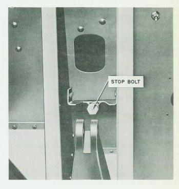
Figure 2-37 Elevator Travel Stop Adjustment
