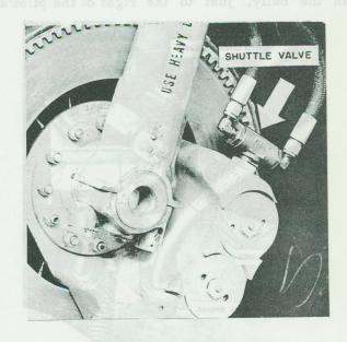
Figure 2-66 Shuttle Valve Mounted on Brakes
