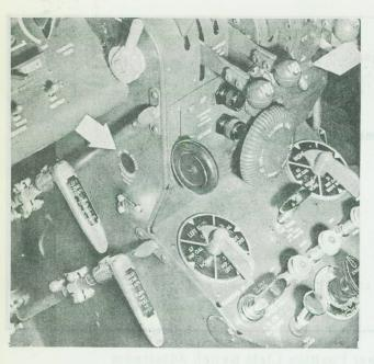
Figure 7-10 Landing Gear Switch Latch Emergency Release
