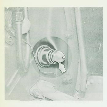
Figure 5-31 Oil Pressure Relief Valve
